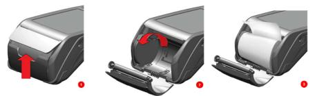
Hold the terminal securely in one hand. With the other hand, and by using two fingers, lift the printer cover release as shown. Fully open the printer cover and remove the old roll of paper.
